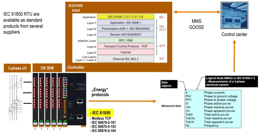
MMS: Manufacturing-Messaging Specifications GOOSE: Generic object oriented substation events
