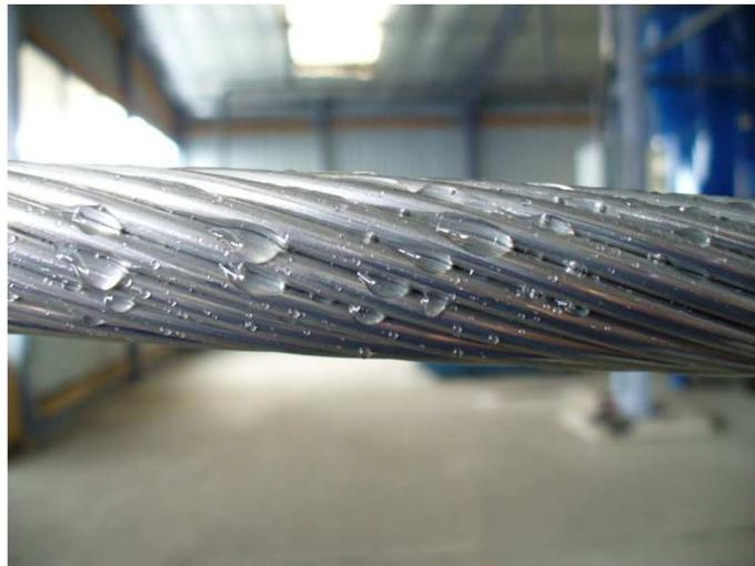
In moisty weather the corona loss is a significant part of the total loss.
